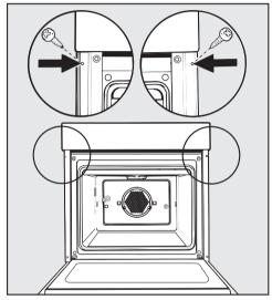
■ Open the oven door and using two screws secure the oven to the side walls of the housing unit through the holes in the oven trim.
